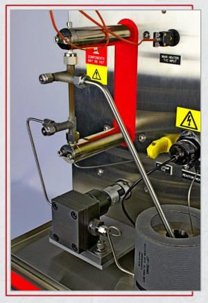
The TEOST™ 33C method has indicated that deposit-formation in the turbocharger is additive-sensitive (additive-free refined mineral base oils of relatively high paraffin content form little deposits by themselves in the TEOST™ 33C). The test has become a required standard for engine oils by OEMs.
