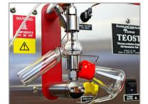
The TEOST™ offers adjustable temperature zones, pump speeds, catalytic materials, and other modification options to simulate desired engine operating conditions.
